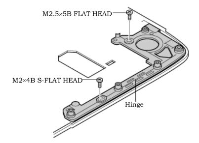
Figure 4-47 Removing the hinge (LCD cable side)
